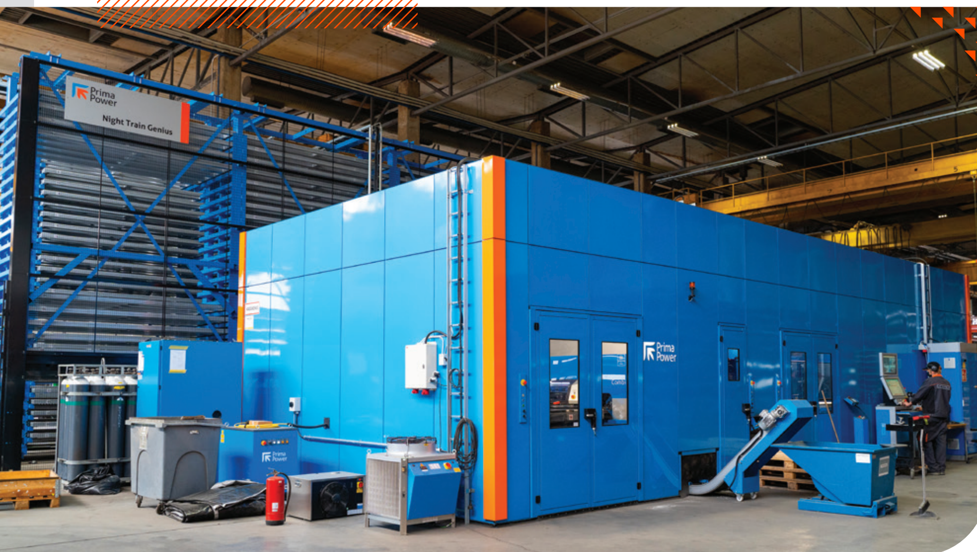
The Combi Genius installed at Lankapaja features an optional protection cabin allowing noise reduction and a more sustainable working environment.
