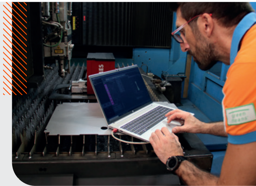
Above Fabio Carantini, Prima Power Field Customer Service Engineer, during a preventive maintenance intervention on the fiber laser head at Rappo.
